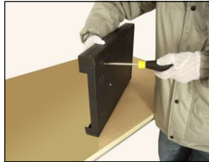
④ Attach hard disk screw
