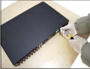
① Remove screws
